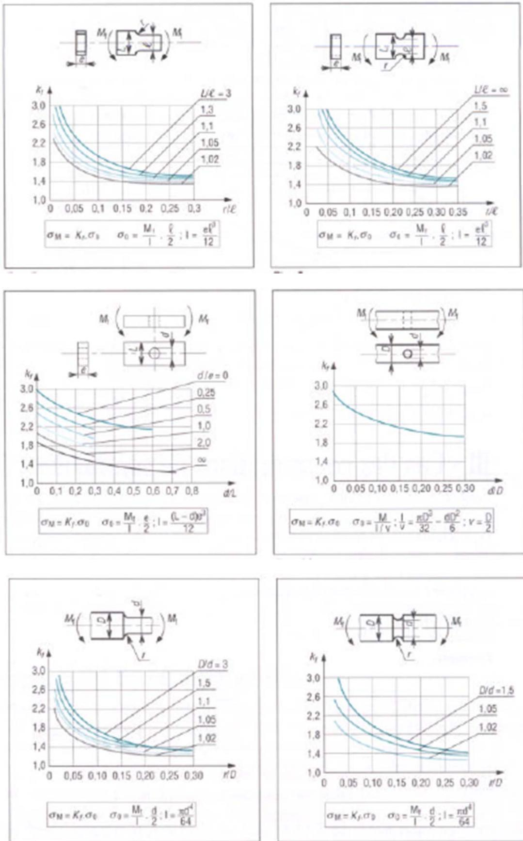
Figure 6.5: Coefficient de concentration de contraintes K en flexion simple.
